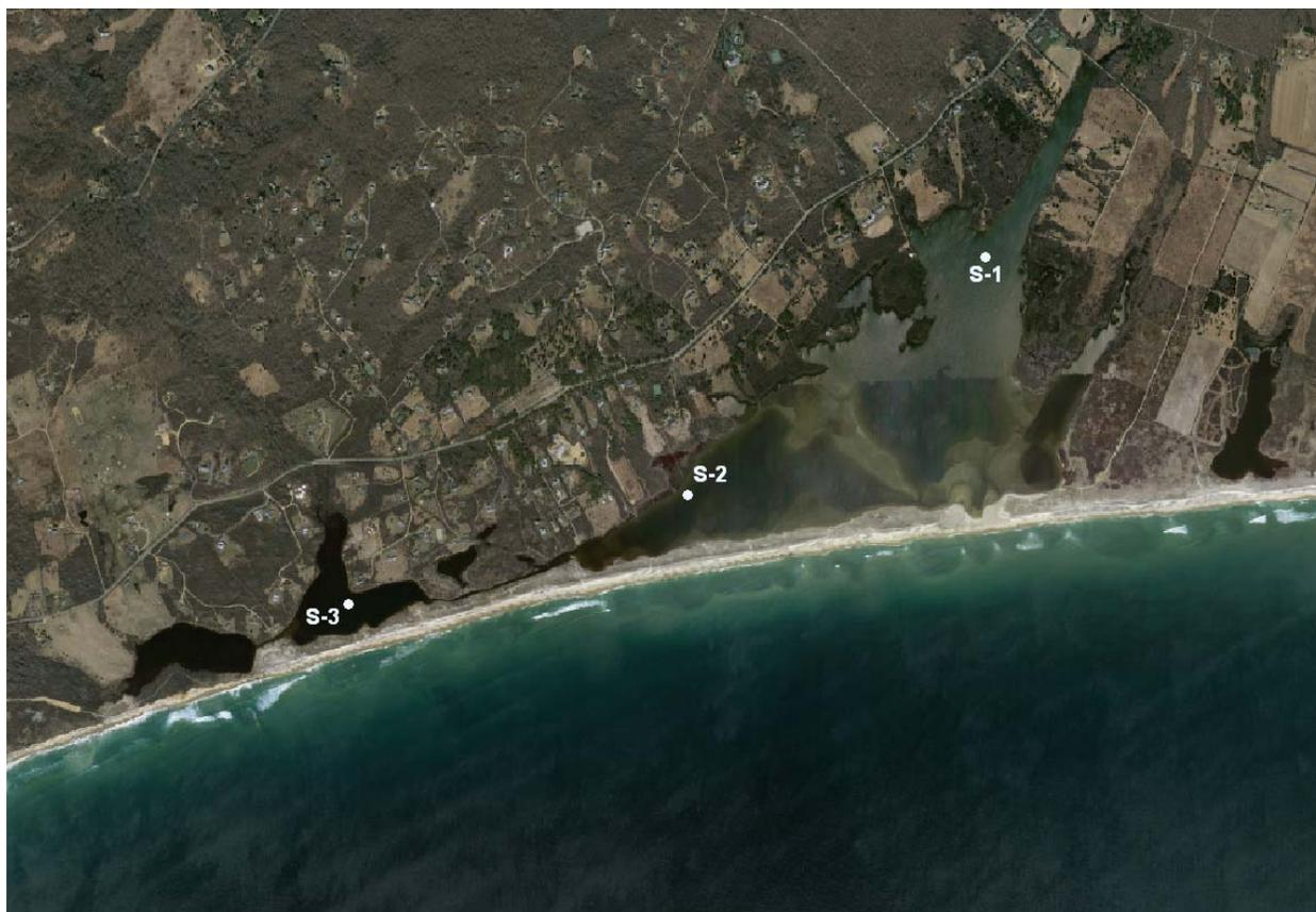
Figure 3. Aerial photograph of the study region identifying locations of the tide gauges used to measure water level variations throughout the system. The gage locations are shown in red: (S-1) represents the north end of the main basin, (S-2) represents the west end of the main basin, and (S-3) represents the sub-embayments to the west.
