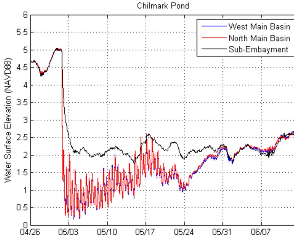
Figure 4. Tide gage signals measured within Chilmark Pond. The figure represents the entire 49-day record (April 26 to June 14 2011). Elevations are referenced to NAVD88.
