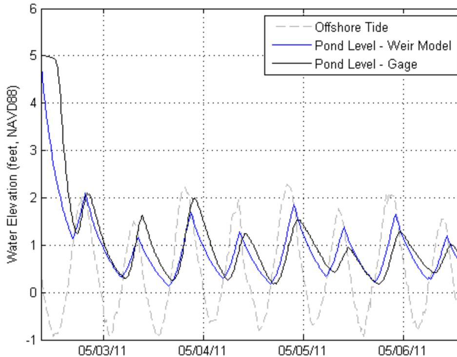
Figure 5. A comparison of the broad-crested weir model results with the recorded pond elevations during the breach event at Chilmark Pond.
