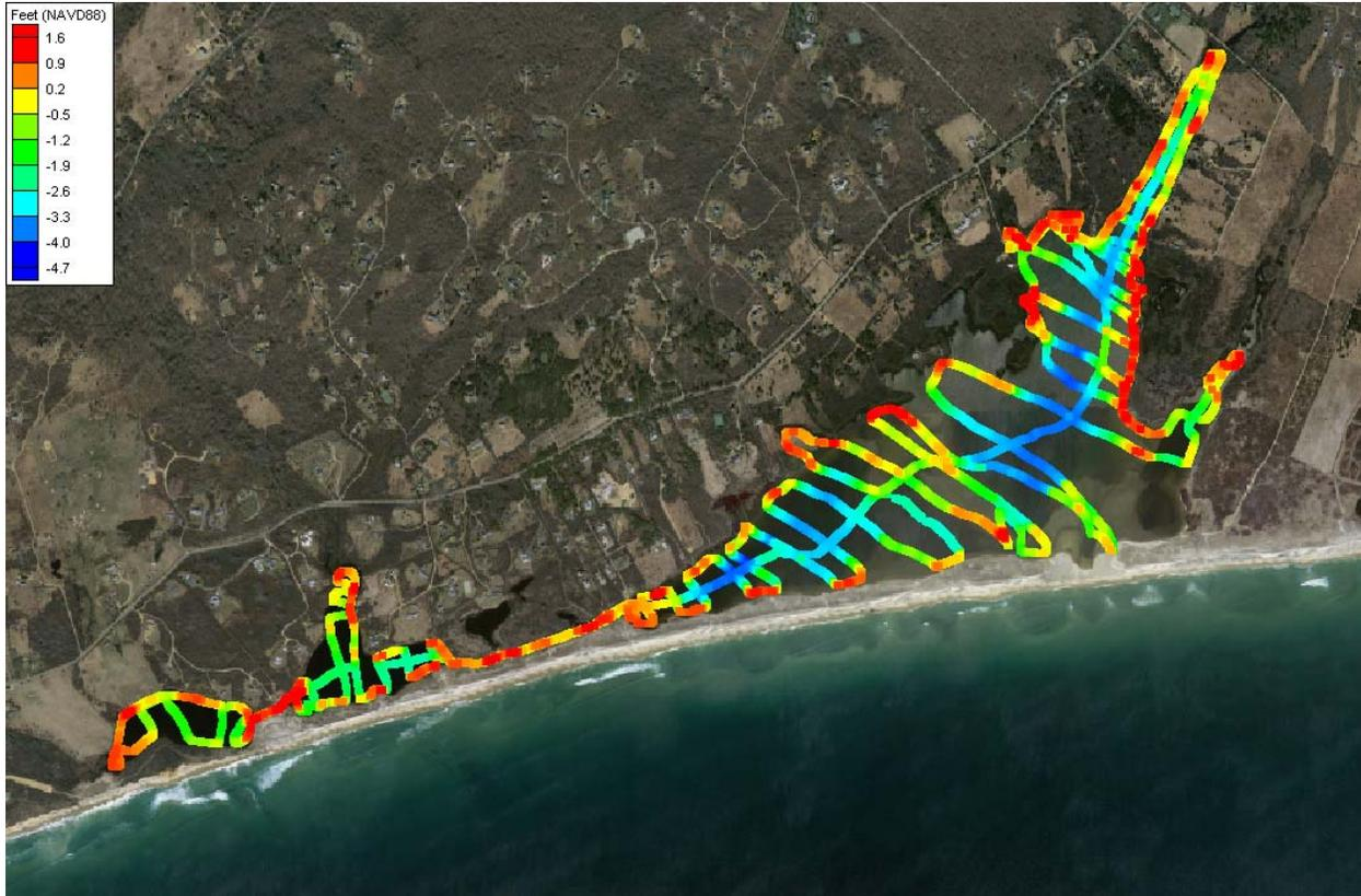
Figure 2. Bathymetry survey lines and depths for Chilmark Pond.
