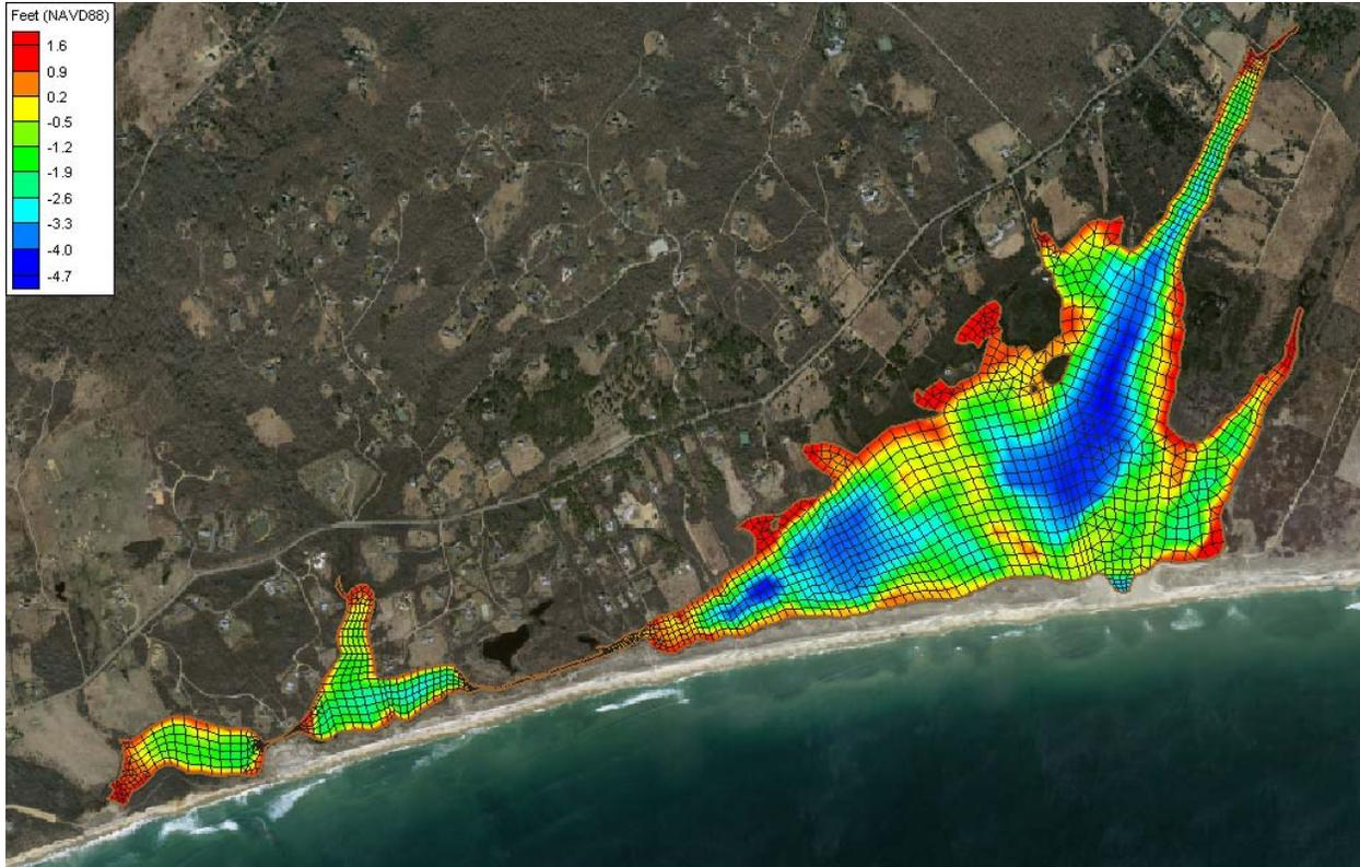
Figure 6. Interpolated bathymetric contours (feet) of the final RMA2 computational mesh of Chilmark Pond. Depth contours are relative to the NAVD88.
